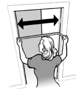
Measuring the clear opening from the face of the doorstop on the frame to the face of the open door.
